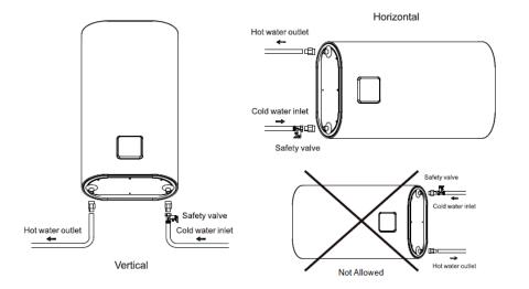
Ants to supply hot water in multiple places, please refer to (Figure4) for pipeline connection and installation. **Note**: When installing the safety valve, be sure to recognize the water flow direction sign on the safety valve and install it correctly, and tighten the upper and lower installation nuts to avoid water leakage. After installation, lift the handle (Figure 5), check whether the safety valve is normal, and then reset.
