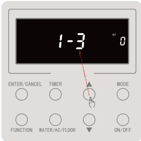
Step 9: Press “▲” or “▼” button to select the sequence (1~6) of shunt valve for setting; Note: If selection is not needed, next step can be entered;
