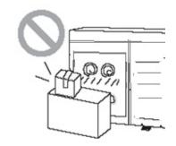
It may reduce efficiency or cause stop of the unit and even fire. Keep pressurized spray, gas holder and so on away from the unit above 1m.
