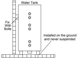
The minimum clearance between the water tank and any combustible object must be 500mm.
