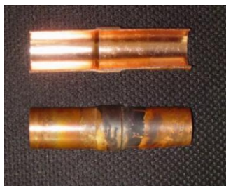
Charge N2 to the pipes
